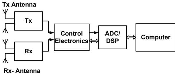
**Figure 3.** The UWB experimental radar structure.
