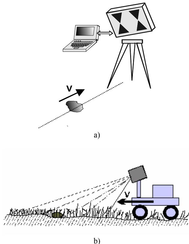
**Figure 2.** Experimental implementation of radar emergency system for two kinds of operation: a) static and b) dynamic.
