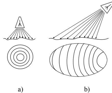
**Figure 1.** Radar's antenna position in accordance to the scene of interest: a) stand-over, b) stand-off.
